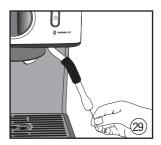
Insert the larger wire into the hole in the base of the steam wand.
